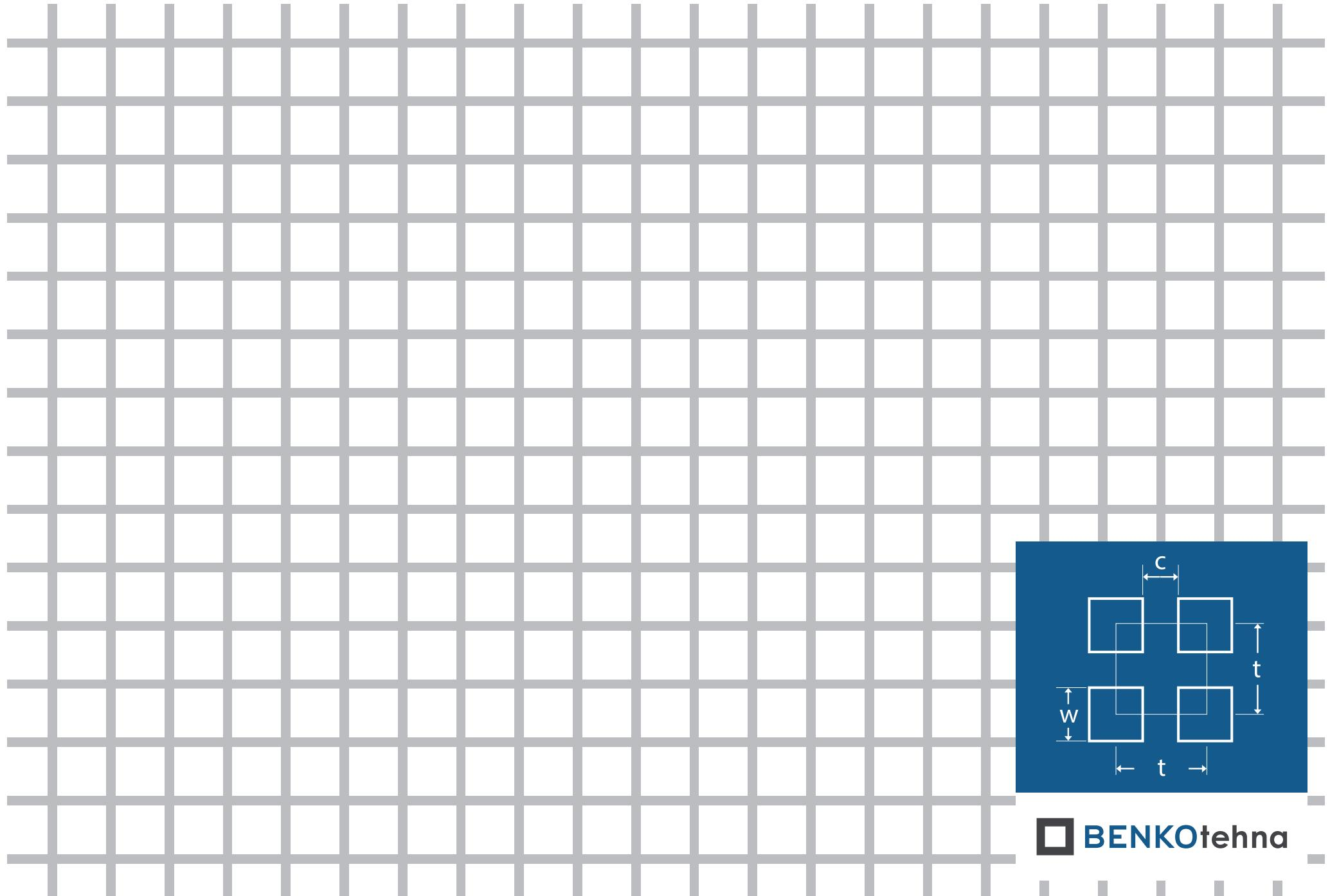
Kvadratna redna Kr 10-12:  $w = 10,0 \text{ mm}$  |  $c = 2,0 \text{ mm}$  |  $t = 12,0 \text{ mm}$  | otvorenost = 69,44%
